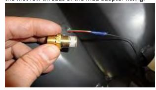
**8.** Install the M12 adapter fitting over the wires and tighten into the fuel tank with a 9/16<sup>-inch</sup> wrench until very tight and about 12mm of the sensor stem can protrude through the fitting when gently lifted.
