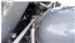
**11.** Disconnect the small 3-pin connector of the low fuel sensor.
