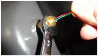
**11.** Cut the old sensor lead wires about 10cm from the connector.
