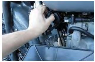
3. Install a piece of hose onto the fuel pump and direct it into a fuel canister.
