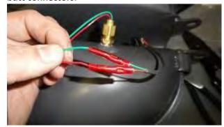
**16.** Wrap the loose wires with a high-quality electrical tape.
