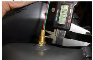
**9.** Hold the sensor in place by lightly pulling up on the wires while you install the compression olive and compression nut.
