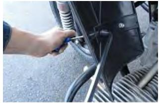
**2.** Remove fuel hose from LH side of the fuel pump.
