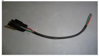
and green-green wires. Crimp with insulated terminal crimping pliers designed for 18-22GA insulated terminals (usually indicated by red mark.) Make sure that both the center metal terminal and outer insulation are crimped creating a mechanical and electrical connection and a water-tight seal. The seal will cure in 3 hours and no heating is required. Lightly tug on the wires to make sure the crimp is mechanically sound. Do not apply heat to the butt connectors.
