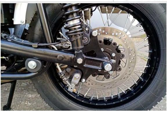
All new rear brake system, utilizing a two-piston Brembo caliper and a standalone mechanical parking brake caliper by J.Juan.
