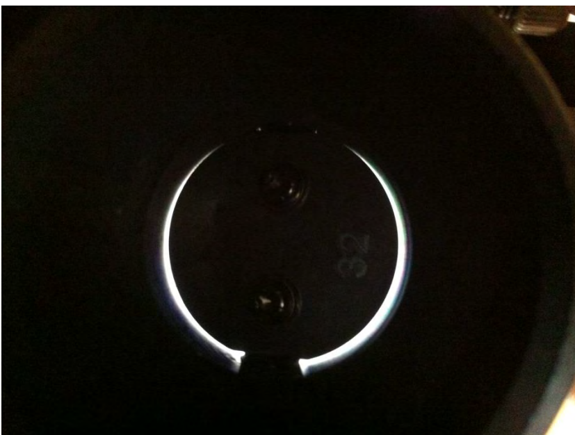
On this picture the gap between the flap and the fuel injection body housing is clear visible. The air can bypass the flap easy which makes it impossible to lower the RPM with the adjustment screw, even with the bell crank spring connected to the correct position.
